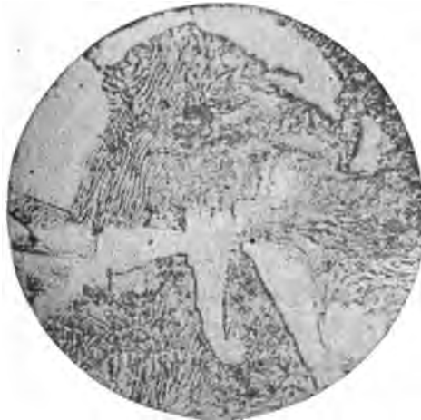
FIG. 46. — White Cast Iron. Magnified 500 Diameters. (Wust.)
